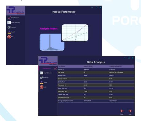
Reporting Functions in Innova Series Porometers: Pore throat diameter, bubble point diameter, mean flow pore size, liquid permeability, pore size distribution, number of pore proportional distribution, cumulative flow distribution, accumulative and differential flow distribution, simultaneous analysis of 12 data files, and overlay for data comparison
