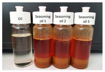
Fig. 3. Seasoning oil samples show an inhomogeneous particle distribution after 2 h 50 min measurement time
