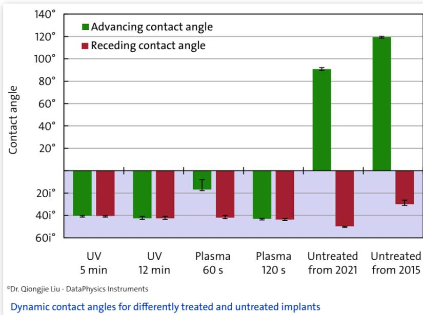
those treated for 12 min (“the gold standard” of implant treatment) are similar, indicating that the treatment time of 5 min could be sufficient regarding wettability. Conversely, the advancing contact angles on implants plasma-treated for 1 min are smaller than those of implants that have been treated for 2 min, suggesting that the treatment time of 1 min is too short to achieve the best possible wetting.
