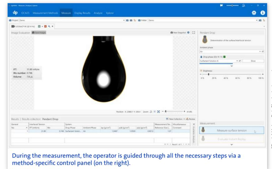
During the measurement, the operator is guided through all the necessary steps via a method-specific control panel (on the right).
