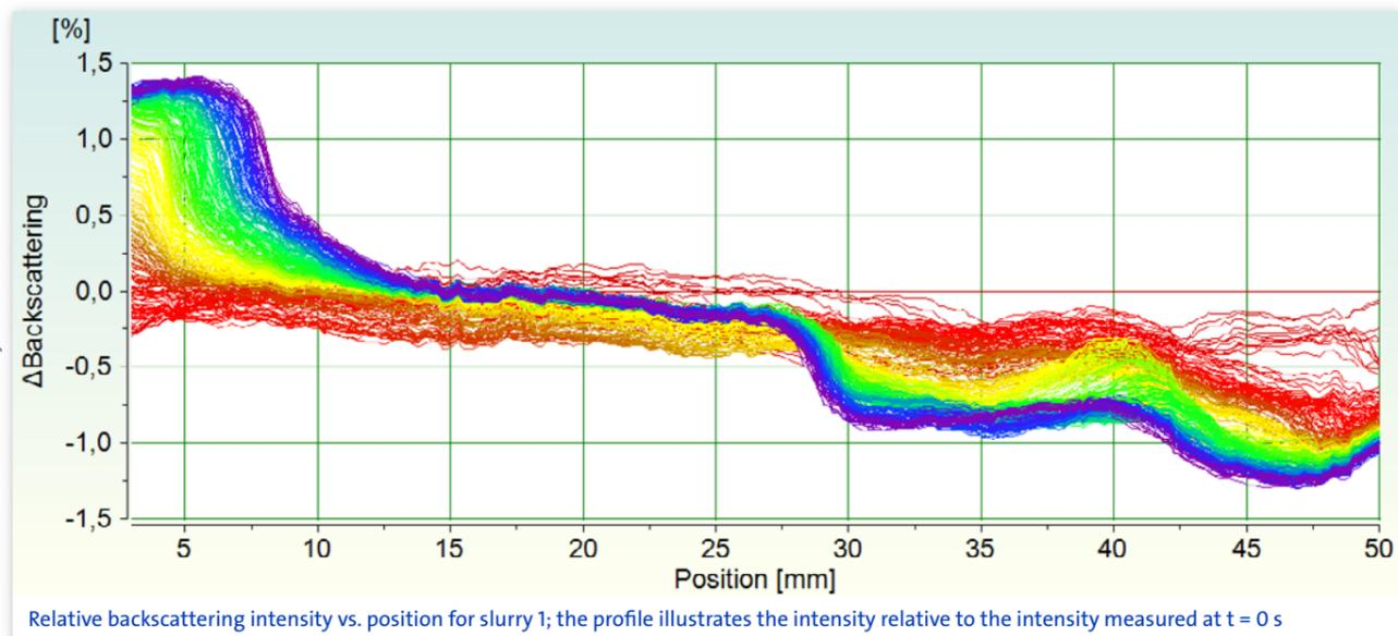
Relative backscattering intensity vs. position for slurry 1; the profile illustrates the intensity relative to the intensity measured at  $t = 0$  s
