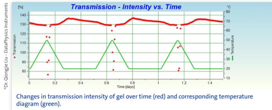
changes within dispersions can be detected and evaluated. The MultiScan MS 20 enables rapid and objective analysis of the dispersion stability as well as conclusions on possible destabilisation mechanisms.
