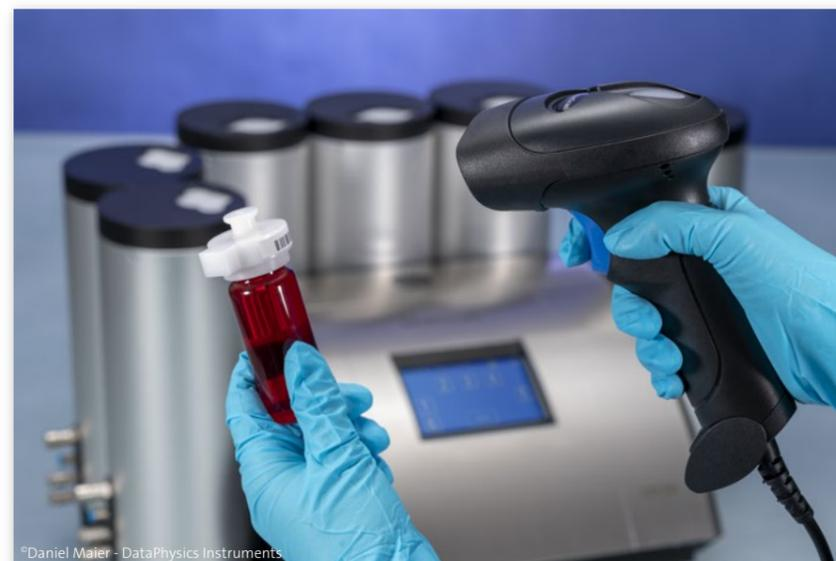
The MultiScan MS 20 dispersion stability analysis system was recently fitted with a handheld scanner to make handling sample containers easier.
