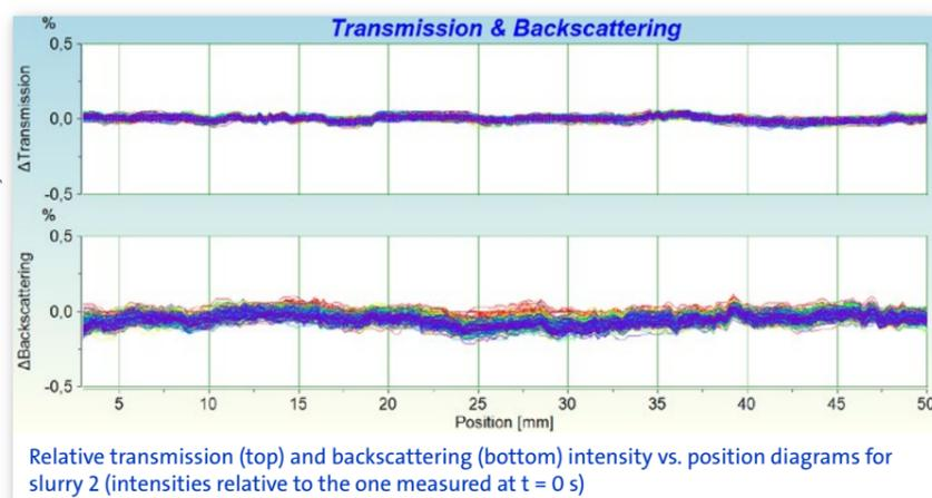
Relative transmission (top) and backscattering (bottom) intensity vs. position diagrams for slurry 2 (intensities relative to the one measured at  $t = 0$  s)
