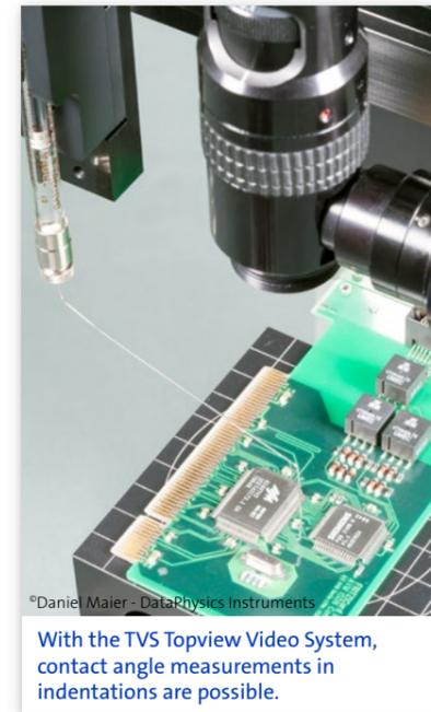
With the TVS Topview Video System, contact angle measurements in indentations are possible.
