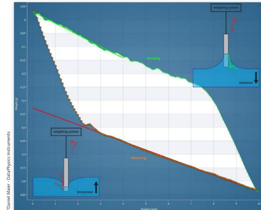
Dynamic contact angles can be measured when the solid sample is dipped in and pulled out of a test liquid. The surface tension of the test liquid must be known.
