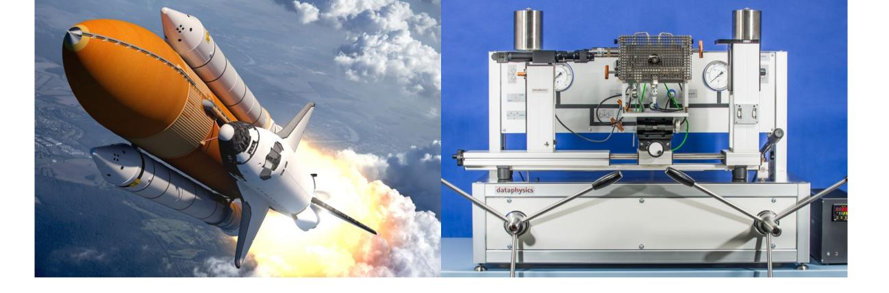
Inside the **high temperature furnace** from DataPhysics Instruments contact angle measurements at up to **1800 °C** and under vacuum down to **10<sup>-5</sup> mbar**, or inert gas atmosphere, are possible.
