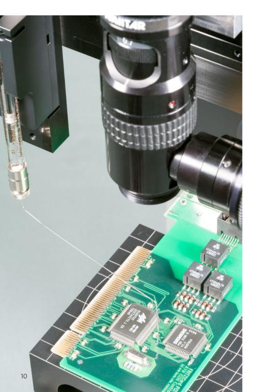
The **Topview Video System TVS** opens up a completely new approach to contact angle measurement. With this system deposited drops are monitored and evaluated in **topview** which allows to investigate previously inaccessible sample spots. Exclusively with the TVS contact angles can be measured, for example, at the bottom of indents of ready-made components or on assembled printed circuit boards.
