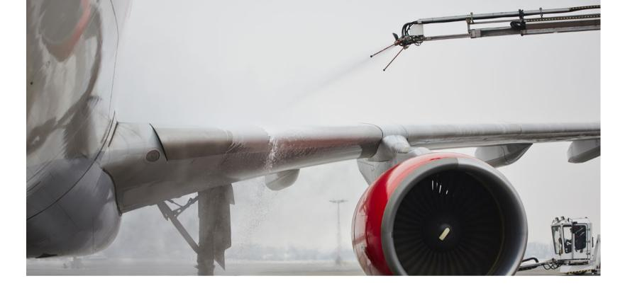
The formation of ice on **airplane wings** influences the aerodynamic properties and the stability of the aircraft. In order to guarantee highest levels of comfort and safety, even at freezing cold temperatures, **de-icing fluids** are used extensively. Their wetting behaviour can be investigated at temperatures of down to -30 °C in a suitable environmental chamber from DataPhysics Instruments.
