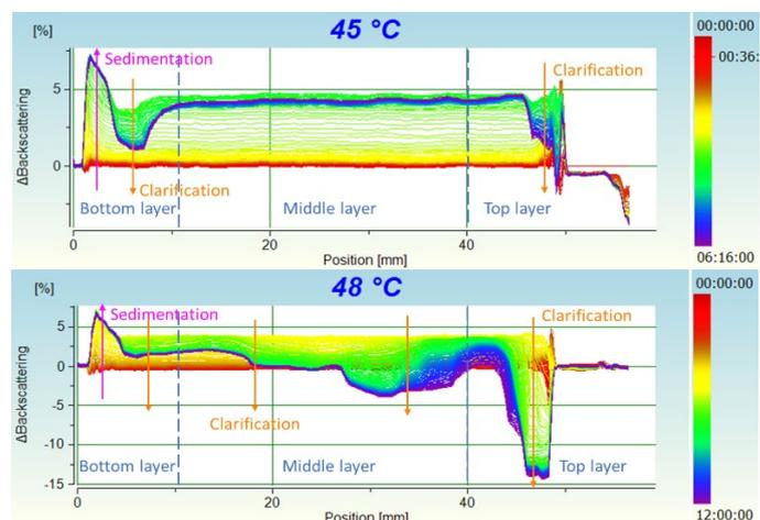
Fig. 6: Backscattering diagram of yogurt formation at 45 °C and 48 °C
