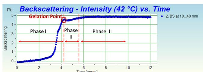
Fig. 5: Kinetics of flocculation in gelation process at 42 °C
