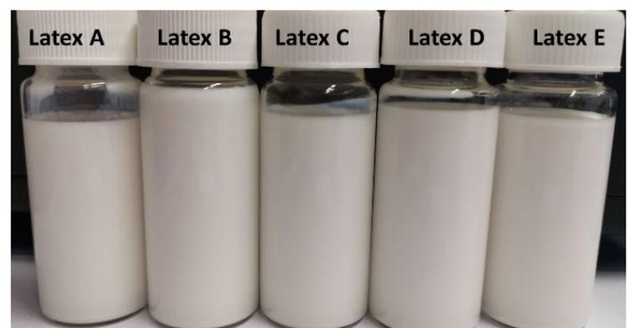
Fig. 3. Samples Latex A, Latex B, Latex C, Latex D and Latex E show a homogeneous particle distribution after 6 days measurement time
