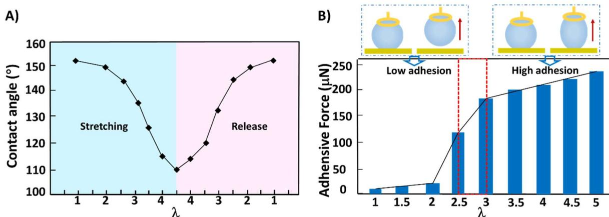
**Figure 2.** A) Reversibly tuneable surface wettability by stretching and releasing the elastomer film from  $\lambda = 1$  to  $\lambda = 4.5$ . B) Dynamic adhesion performance of the micro/nanostructured elastomer film with varying stretch ratios ( $\lambda$ ).
