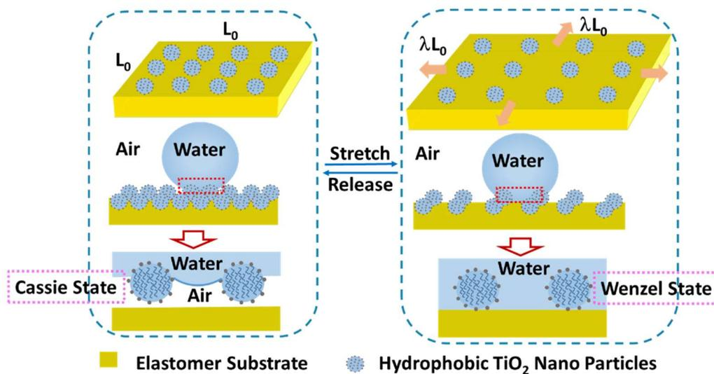
**Figure 1.** Controllable wettability of elastomer films by adjusting the space of micro/nano-structured clusters of  $\text{TiO}_2$  nanoparticles on the surface through stretching.
