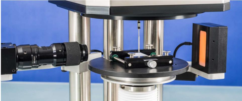
This system combines a force measurement to determine the force of adhesion and an optical system to determine the area of contact between the liquid/gas and solid phase for each force that is measured. Like this a force per area can be determined. The measurement procedure involves a liquid or gas bubble being pushed onto a solid substrate under air or liquid and being pulled off from it again.
