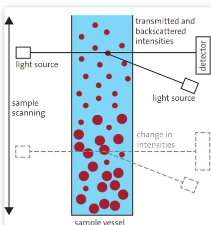
Fig. 2: MultiScan measuring principle
