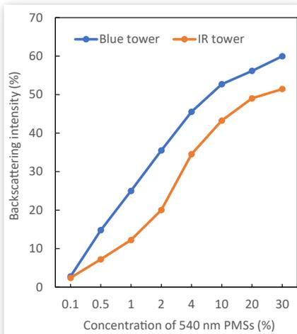
**Fig. 6: The backscattering intensity of 540 nm PMSs with different volume concentrations measured by Blue tower and IR tower, respectively**
