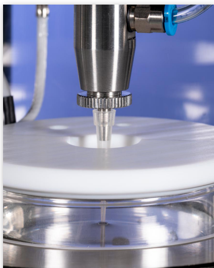
Fig. 3: Disposable capillaries utilised in MBP 200 with PTFE cover
