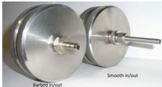
Triple flange with gas in/out nozzles
