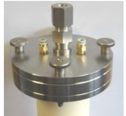
Triple flange end seal with thermocouple gland
