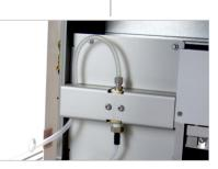
The vacuum assisted waste stream prevents blockages when processing viscous samples.
