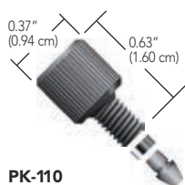
PK-110 10-32 PK Fitting shown with PK-100 for 1/16" OD tubing
