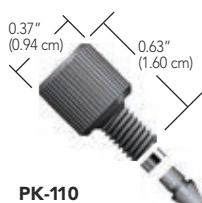
PK-110 10-32 PK Fitting shown with PK-132 for 1/32" OD tubing
