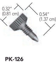
PK-126 6-32 PK MicroTight® Fitting for 1/32" OD tubing
