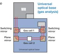
A wide range of gas concentrations can be applied by attaching gas cells with several different pathlengths.
