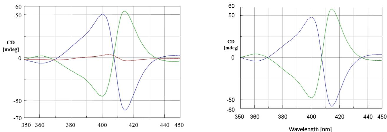
**Figure 4.** MCD spectra of Fe(III) cytochrome c before (left) and after (right) subtraction of the CD spectrum. The blue spectra show the magnetic field in the forward direction, the green illustrate the magnetic field in the reverse direction, and red spectra are in the absence of a magnetic field.
