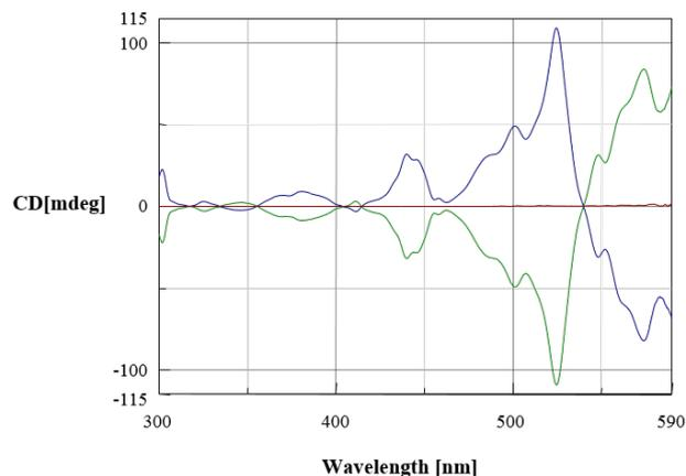
**Figure 6.** MCD spectra of cobalt chloride (II) 6 hydrate in concentrated hydrochloric acid solution. The blue spectra show the magnetic field in the forward direction, the green illustrate the magnetic field in the reverse direction, and red spectra are in the absence of a magnetic field.
