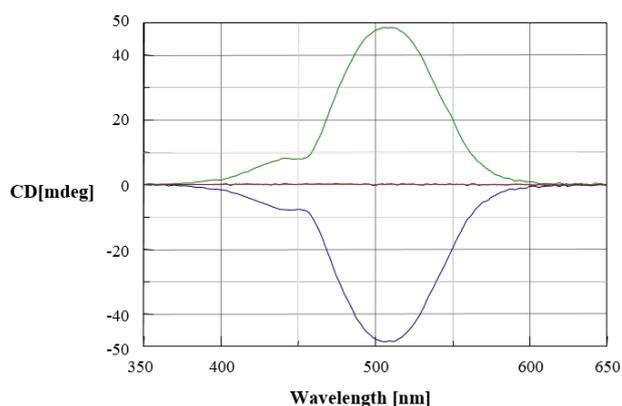
**Figure 5.** MCD spectra of cobalt chloride (II) 6 hydrate in aqueous solution. The blue spectra show the magnetic field in the forward direction, the green illustrate the magnetic field in the reverse direction, and red spectra are in the absence of a magnetic field.
