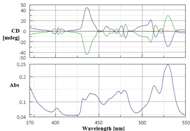
**Figure 2.** MCD (top) and absorption (bottom) spectra of neodymium glass in the UV-Vis region. The blue spectra show the magnetic field in the forward direction, the green illustrate the magnetic field in the reverse direction, and red spectra are in the absence of a magnetic field.
