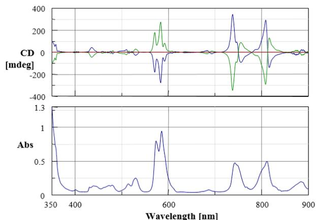
**Figure 1.** MCD (top) and absorption (bottom) spectra of neodymium glass in the NIR region. The blue spectra show the magnetic field in the forward direction, the green illustrate the magnetic field in the reverse direction, and red spectra are in the absence of a magnetic field.
