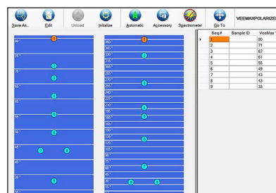
AutoPRO Software control of VeeMAX III angle of incidence (automated polarizer available) for automated depth profiling studies, angle of incidence and polarization angle can be set independently.
