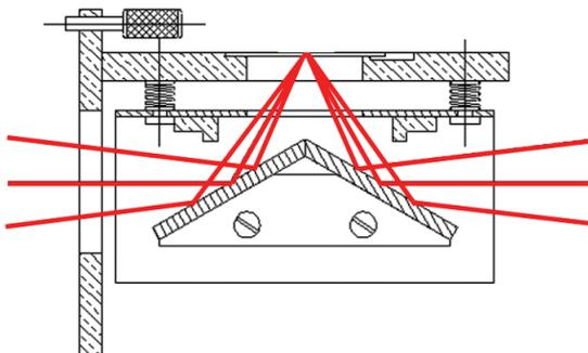
Optical geometry for the 30Spec.
