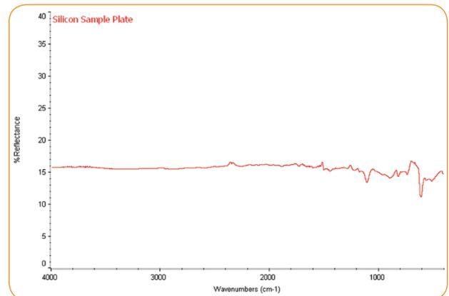
Spectrum of a silicon plate measured in the PIKE Absolute Reflectance Accessory.
