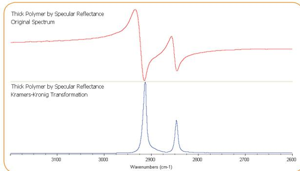
*Spectrum (upper – original) of a relatively thick polymer sample measured at 30 degrees angle of incidence using the VeeMAX III; the lower spectrum has been transformed using the Kramers-Kronig software algorithm and is very similar to a transmission spectrum of the polymer polyethylene.*
