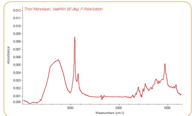
*Grazing angle specular reflection analysis of a thiol mono-molecular layer deposited on a gold-surfaced mirror using the PIKE VeeMAX III at 80 degrees and p-polarization; the FTIR was equipped with an MCT detector.*
