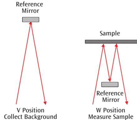
Beam path for V and W positions for the PIKE Absolute Reflectance Accessory.
