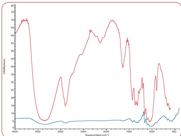
Comparison of transmission spectrum of paper collected using an integrating sphere or in transmission mode without a sphere.
