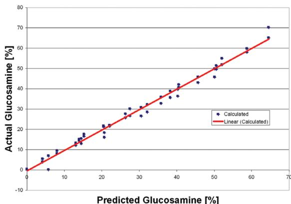
Quantitative measurement of active ingredient in a mixture of magnesium stearate, lactose, EMCOMPRESS®, cellulose and CAB-O-SIL®
