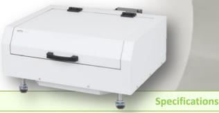
The ARSV-916 accessory provides absolute reflectance measurements of samples by the manual, asynchronous movement of the sample stage and detector, thus, the positions of the sample stage and detector can be independently varied to obtain the absolute reflectance and transmittance spectra of the sample at varied incident and detection angles.
