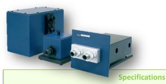
FAV-750 accessory consisting of an optical fiber unit and external detector, enables the measurement of bulky samples that cannot be set in the sample compartment and/or samples that are in special environments. The light from the main instrument is introduced to the optical fiber. The light from a sample is introduced to the external detector via the optical fiber.
