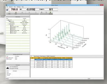
**Validation** - V-750 provides a standard validation program. This program supports USP, EP and JP instrument qualification requirements. The program automatically performs an analysis of the instrument results based on defined acceptance criteria. Results of the validation tests can be printed or saved electronically for further review.
