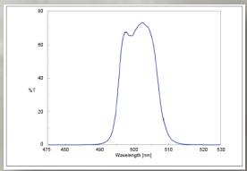
Transmittance Spectrum of Bandpass Filter
