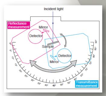
The ARMV-919 automates the absolute reflectance measurements of specularly reflecting samples such as metal or glass samples. The detector is equipped with an integrating sphere and thus it also permits measurement of the relative reflectance of a diffusely reflecting sample. Since the angles of the sample stage and the detector can be changed independently, the absolute reflectance and transmittance of a sample can be measured with varied angles of incidence.
