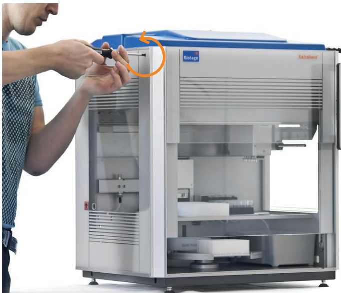
Figure 9. Open the door manually by turning the screw counterclockwise.
