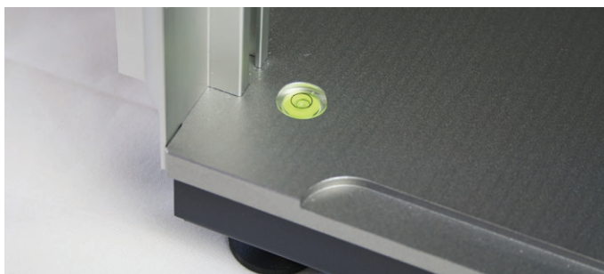
Figure 2. The built-in spirit level in the bottom of the system, in the front left corner.
