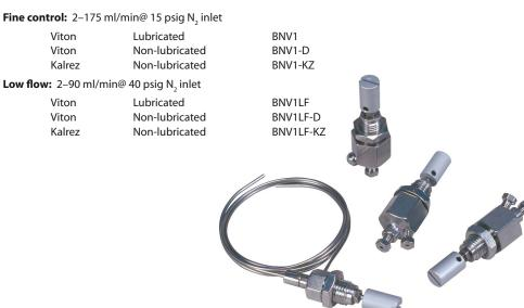
VICI regulators are machined from aluminum bar stock and then hardanodized to provide contaminationfree service. They feature a stainless steel diaphragm and Viton®-sealed stainless poppet. The compact size (1.125" diameter by 2" long for regulator, 3" long for combo version) saves panel space and permits installation anywhere that an 11/16" hole can be located. Mounting hardware is supplied.
