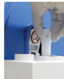
Insert the vial using the vial loading tool.
