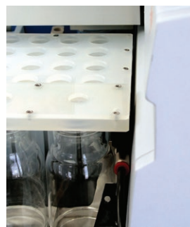
Cover plates placed to depress gas nozzles on an Inert Gas Manifold, allowing gas to flow.
