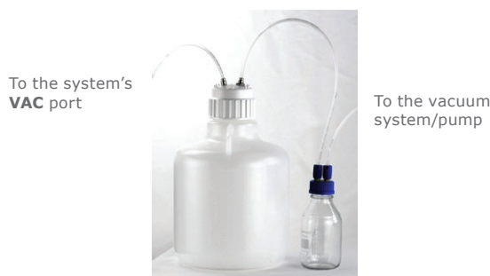
The waste & scrubber kit contains a 10 liter waste reservoir, a 0.5 liter scrubber bottle, and the tubing shown above.
