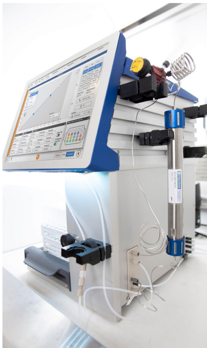
Figure 2. The semi-preparative HPLC column setup on Biotage® Selekt.
