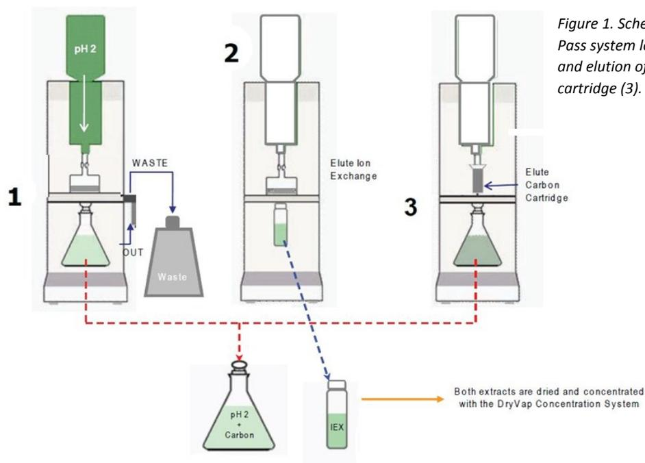
Figure 1. Schematic of the One-Pass system loading of sample (1) and elution of the disk (1,2) and cartridge (3).
