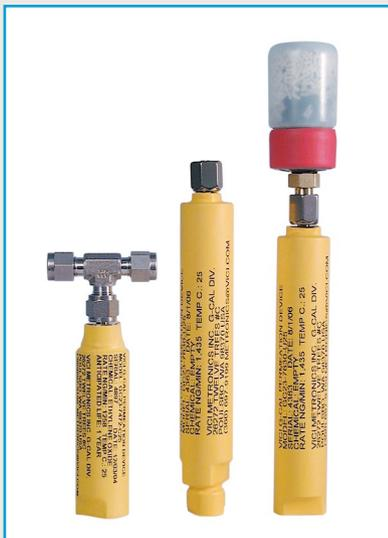
Over 100 different substances are available, including Arsine, Phosphine, and gas phase devices such as CO, NO, and Methane. Available permeation rates range from less than 100 ng/min to 50,000 ng/min. Each G-Cal device is individually calibrated and verified to generate a given mass output per unit time (ng/min) at a set point temperature. A graph which shows an estimated permeation rate vs. temperature from 0 to 50°C is included with each device.
