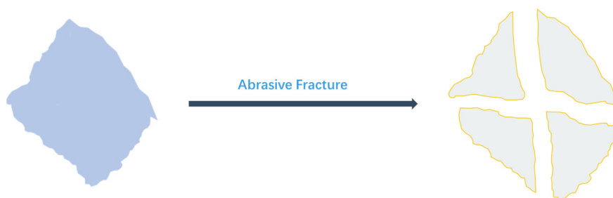
Figure 1. Diagram of self-sharpening behavior of abrasives
