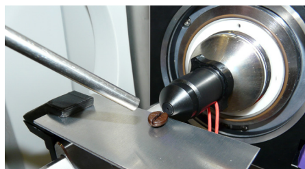
Figure 2 - Coffee aroma profiling by direct VOC desorption in front of the SICRIT ® ion source.
