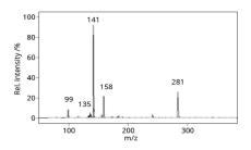
Figure 3 - Full SICRIT® mass spectrum of sarin with M+H (m/z 141), M-C<sub>3</sub>H<sub>6</sub> (m/z99), M+H<sub>2</sub>O (m/z 158) and 2M+H (m/z 281) species acquired on the AB Sciex MS.
