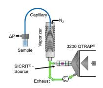
Figure 2 - Schematic sketch of the setup using the AB Sciex benchtop  $\ensuremath{\mathsf{MS}}.$
